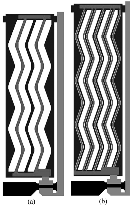
FIGURE 1 Liquid crystal display cell configuration: (a) conventional S-IPS cell and (b) proposed high transmittance S-IPS cell (Case 2).
